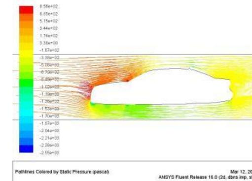
Picture showing static pressure of hatchback mid model 1 mid at 80kmph
