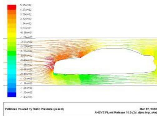
Picture showing static pressure of hatchback model 1 front at 60kmph
