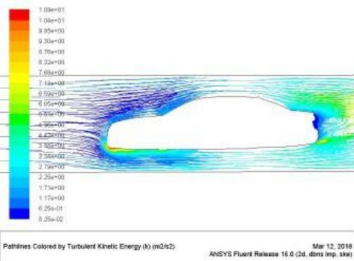
Picture showing turbulent kinetic energy of hatchback model 1 rear at 60kmph
