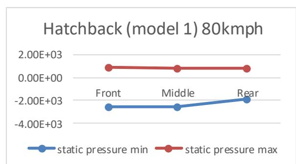
Graph showing static pressure for hatchback Model 80kmph
