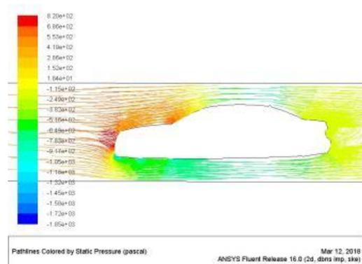
Picture showing static pressure of hatchback model 1 rear at 80kmph
