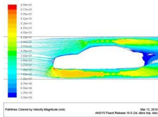
Picture showing velocity magnitude of hatchback model 1 front at 80kmph
