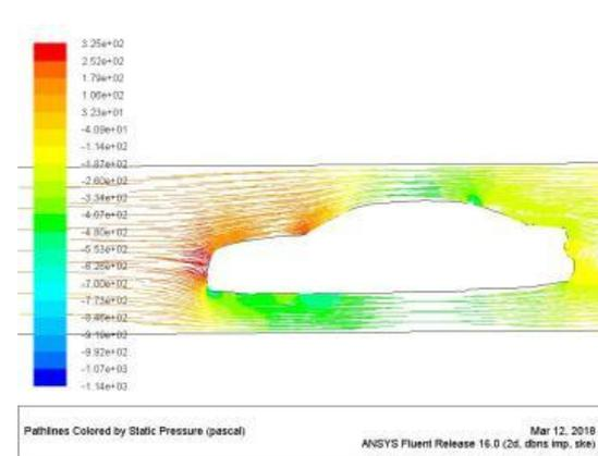
Picture showing static pressure of sedan class model 1 rear at 60kmph
