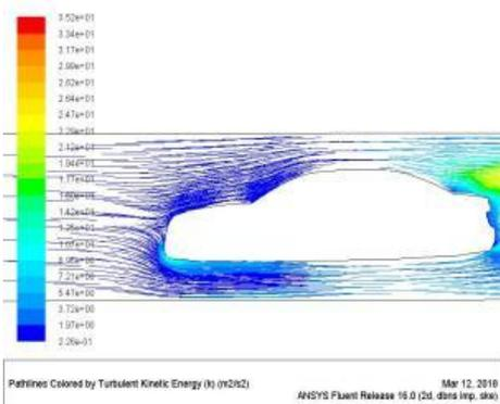
Picture showing turbulent kinetic energy of Hatch back model 1 front at 60kmph
