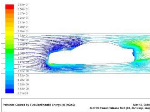
Picture showing turbulent kinetic energy of hatchback model 1 mid at 80kmph
