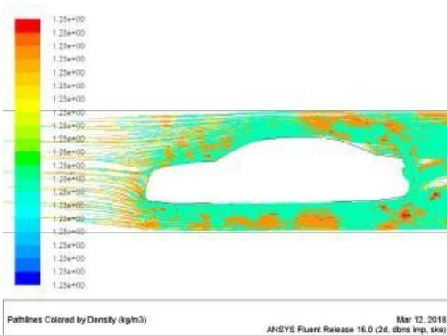
Picture showing density of hatchback model 1 front at 80kmph
