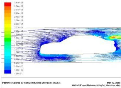
Picture showing turbulent kinetic energy of sedan class model 1 rear at 60kmph
