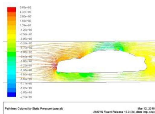
Picture showing static pressure of sedan class model 1 mid at 80kmph
