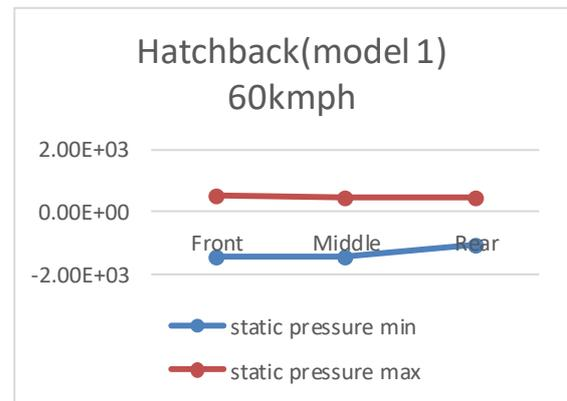
Graph showing static pressure for hatchback model 1 at 60kmph
