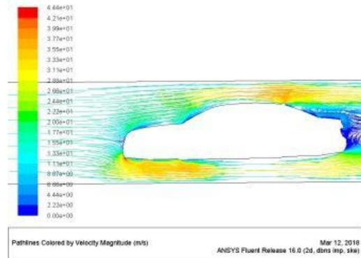
Picture showing velocity magnitude of sedan class model 1 rear at 60kmph
