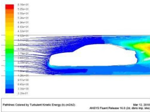
Picture showing turbulent kinetic energy of hatch back model 1 front at 80kmph
