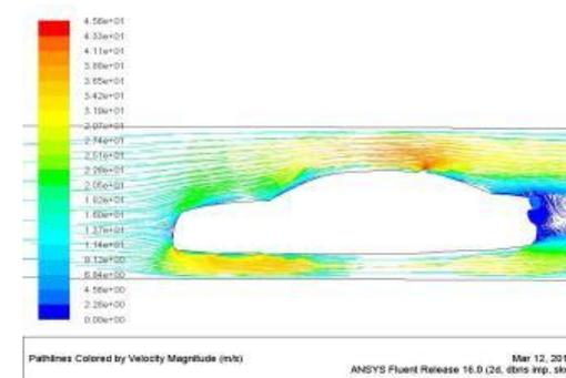
Picture showing velocity magnitude of sedan class model 1 fronts at 60kmph
