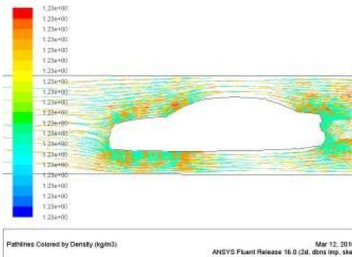
Picture showing density of hatchback model 1 rear at 80kmph
