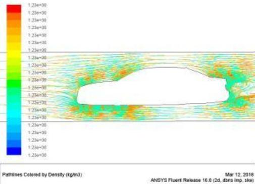
Picture showing density of hatchback model 1 rear at 60kmph
