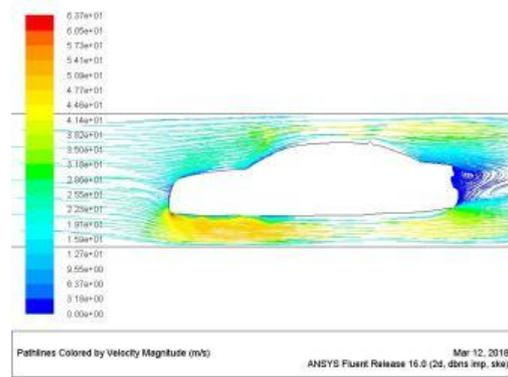
Picture showing velocity magnitude of hatchback model 1 mid at 80kmph
