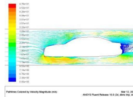
Picture showing velocity magnitude of hatch back model 1mid at 60kmph
