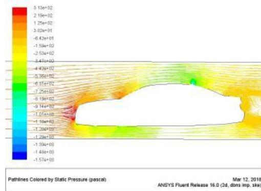
Picture showing static pressure of sedan Class model 1 front at 60kmph
