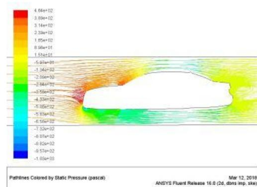
Picture showing static pressure of hatchback model 1 rear at 60 kmph
