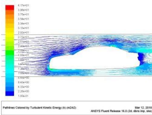
Picture showing turbulent kinetic energy of sedan class model 1 front at 80kmph
