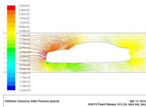
Picture showing static pressure of hatchback model 1 mid at 60kmph
