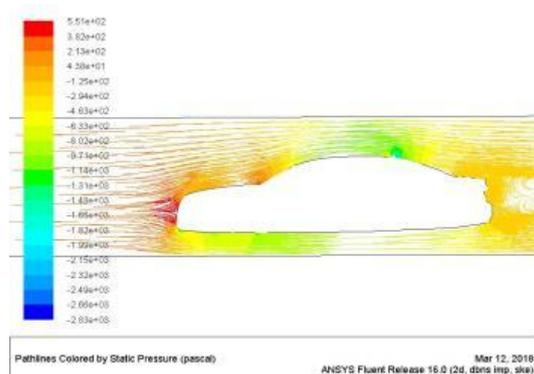
Picture showing static pressure of sedan class model 1 front at 80kmph
