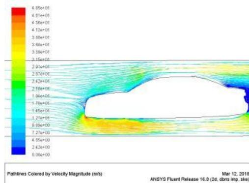
Picture showing velocity magnitude of hatchback model 1 front at 60kmph
