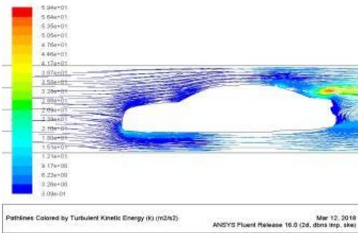
Picture showing turbulent kinetic energy of sedan class model 1 rear at 80kmph
