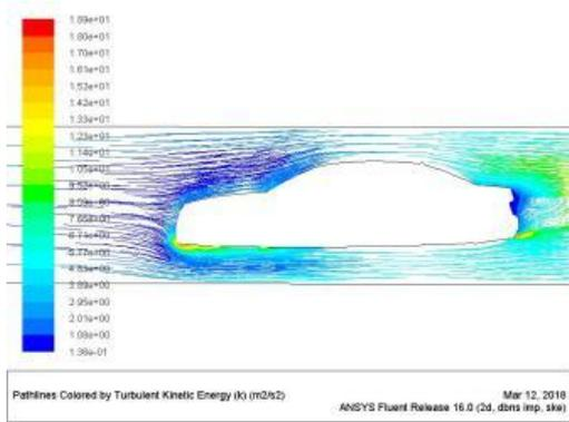
Picture showing turbulent kinetic energy of hatchback model 1 rear at 80kmph
