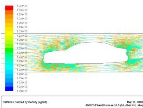
Picture showing density of hatchback model 1 mid at 60kmph
