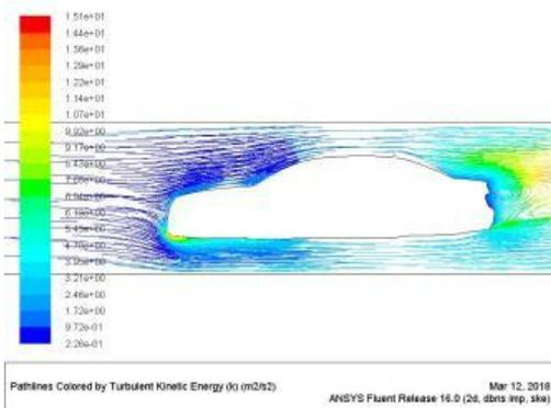
Picture showing turbulent kinetic energy of hatchback model 1mid at 60kmph
