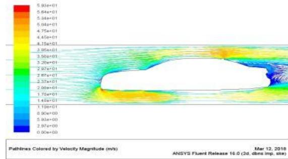
Picture showing velocity magnitude of sedan class model 1 rear at 80kmph
