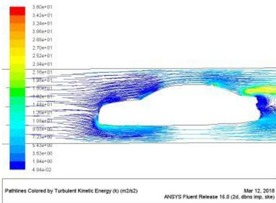
Picture showing turbulent kinetic energy of sedan class model 1 mid at 80kmph
