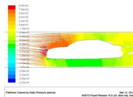
Picture showing static pressure of hatchback model 1 front at 80kmph
