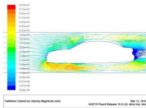
Picture showing velocity magnitude of hatchback model 1 rear at 80kmph
