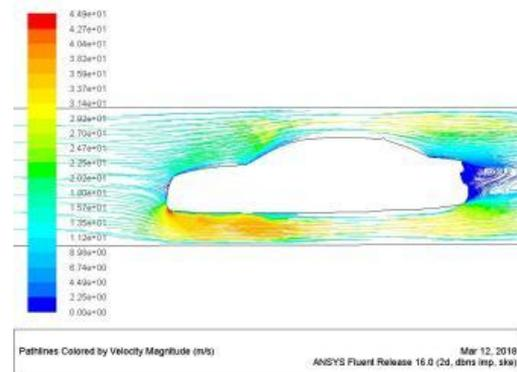
Picture showing velocity magnitude of hatchback model 1 rear at 60kmph
