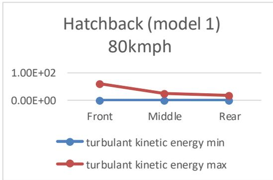
Graph showing turbulent kinetic energy for hatchback model 1 at 80kmph
