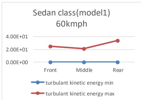
Graph showing turbulent kinetic energy for sedan class model 1 at 60kmph
