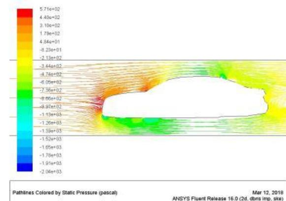
Picture showing static pressure of sedan class model 1 rear at 80kmph
