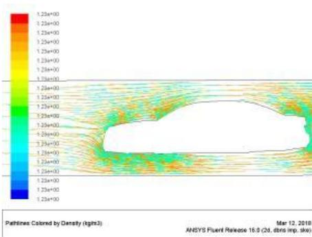
Picture showing density of hatchback model 1 front at 60kmph
