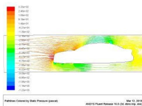
Picture showing static pressure of sedan class model 1 mid at 60kmph
