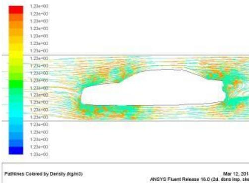
Picture showing density of hatchback model 1 at 80kmph
