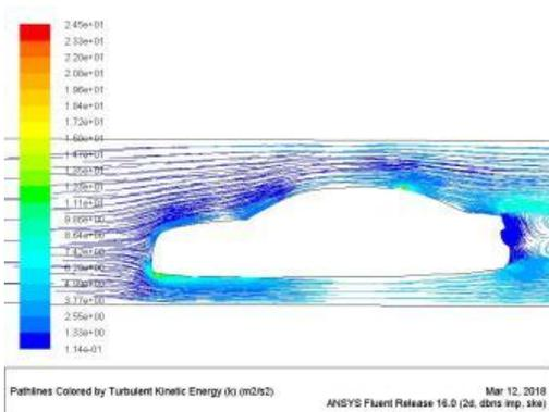
Picture showing turbulent kinetic energy of sedan Class model front at 60kmph
