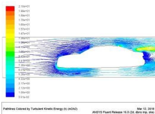
Picture showing turbulent kinetic energy of sedan class model 1 mid at 60kmph
