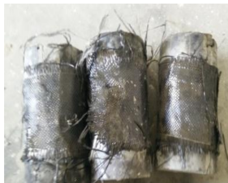
Fig-2: CFRP Sheet wrapped on concrete
