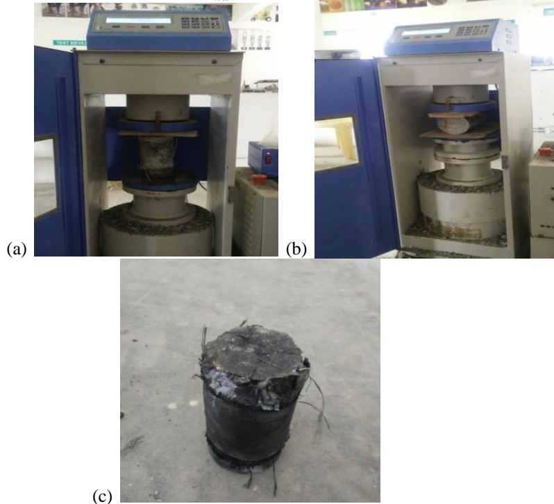
Fig-3: (a) Compression strength test (b) Split-Tensile Test (c) Tested sample specimen
