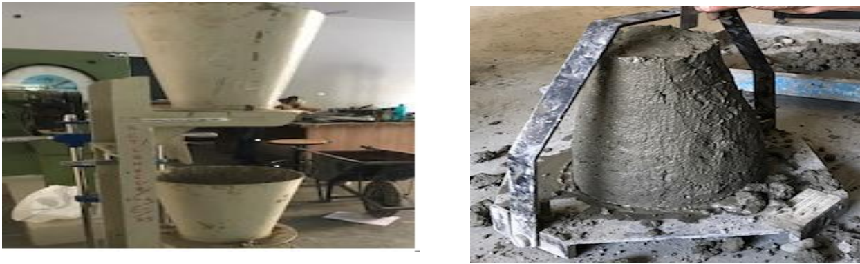
Fig 1: Compacting factor test and slump cone test of fresh concrete
