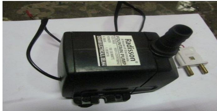
Fig. 9. Water Circulation pump
