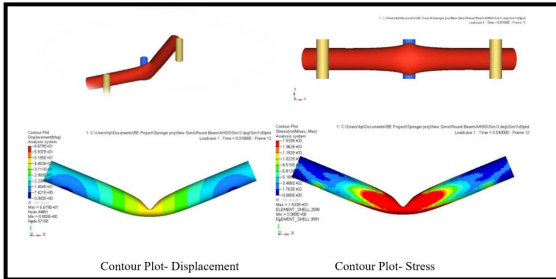
Fig. 6 Results for Circular beam / AHSS / 0 degrees
