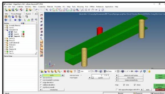
Fig. 5 C-section hollow beam meshing
