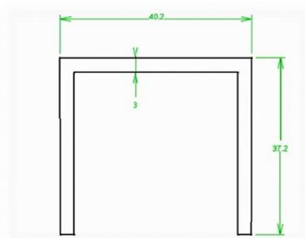
Fig.1 C-section beam dimensions
