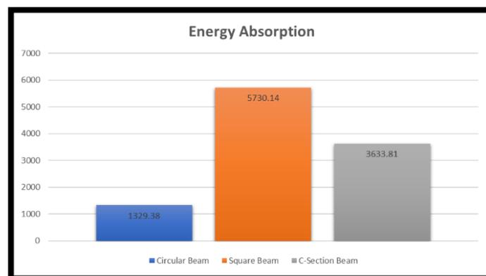
Fig. 8 Maximum Energy Absorption classified according to cross-section of beam
