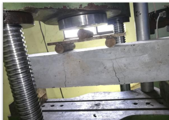
Fig.3 Testing of Retrofitted Beam
