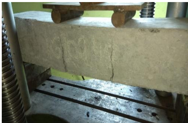
Fig.2 Testing of RC Beam
