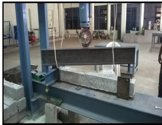
Fig: Typical failure of the specimen under torsion
