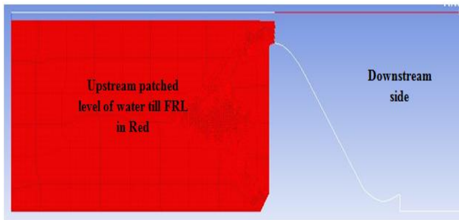
Fig. 5 Patched Water Level
