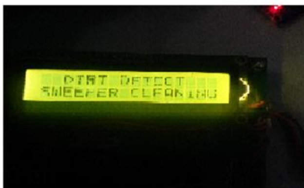
Figure 1.12: Output module, while detecting the dirt
