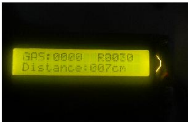
Figure 1.13: Output module, while detecting the Gas and the distance.
