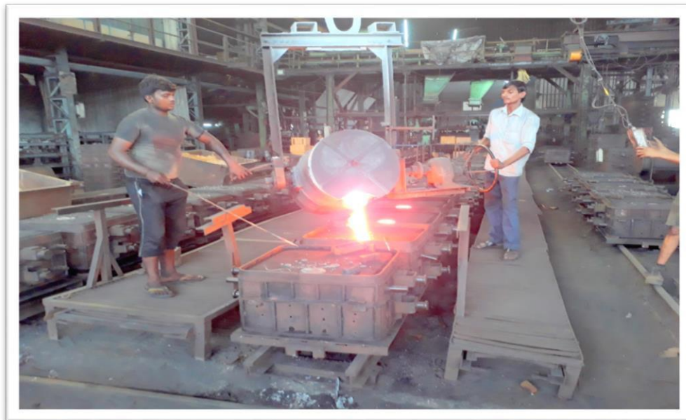
[Fig.1 pouring process]
