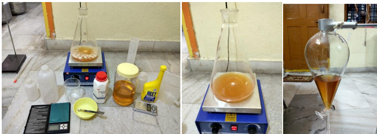
Fig 4: Laboratory biodiesel preparation steps (a) methyl Alcohol (CH 3 OH) and catalyst potassium hydroxide (KOH) at various wt% (weight percent) are mixed together.
