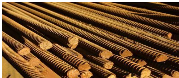
(d) : Absolutely fresh ribbed TMT bars stacked at the factory before despatch, showing onset of corrosion all over the surface
