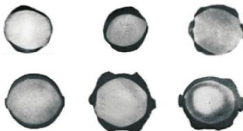
(a) : Non-uniform quenching of TMT bars
