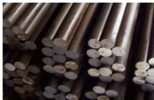
(g) : Conventional rebars with plain surface as used to be used decades earlier; also as in PSWC bar
