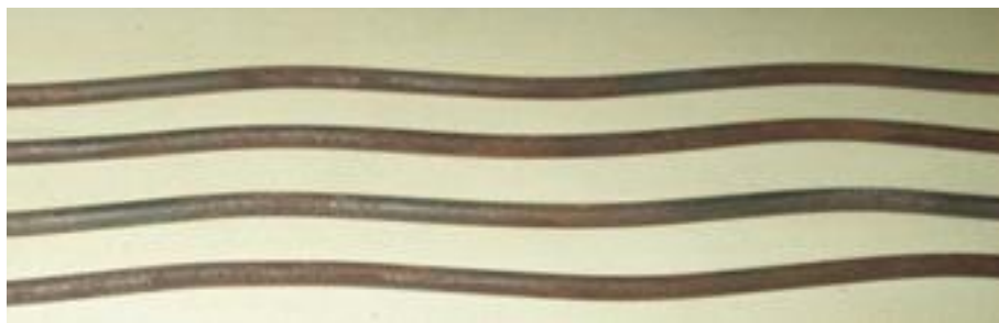
(a) : Elegant PSWC bars characterized by plain surface and gentle wave- type configuration (photograph of actual bars)
