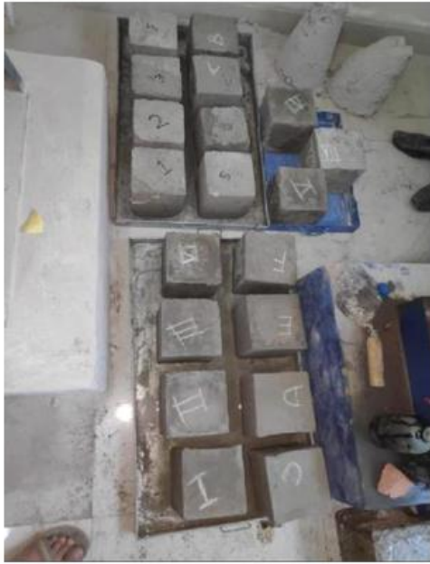
CLC blocks after remoulding
