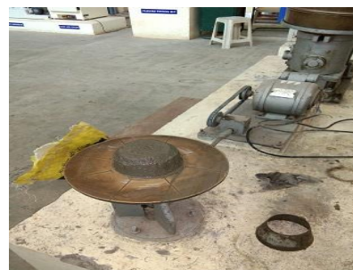
Fig.4 Placing of bottom ash cement mortar in flow table mould
