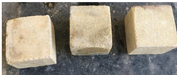
Fig. 12 Acid Attack Mortar Cubes Specimens in 14, 28 and 60 days
