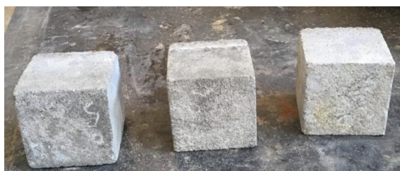
Fig. 14 Salt Attack Mortar Cube Specimens in 14, 28 and 60 days
