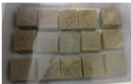
Fig. 13 Mortar Cubes Specimens Immersed in Sodium Chloride
