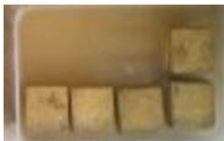
Fig. 11 Mortar Cubes Specimens Immersed in H 2 SO 4
