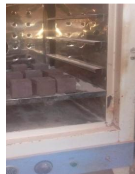
Fig. 7 Oven at 105°C Temperature on Specimens
