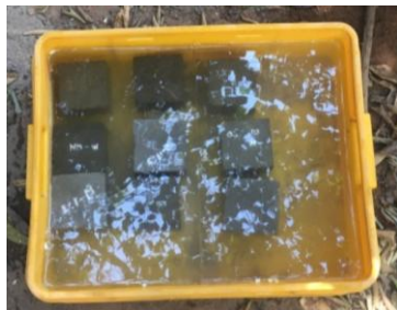
Fig.6 Curing of Mortar Specimen for Water Absorption
