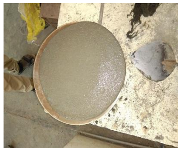
Fig.5 Shape of mortar mix after flow test
