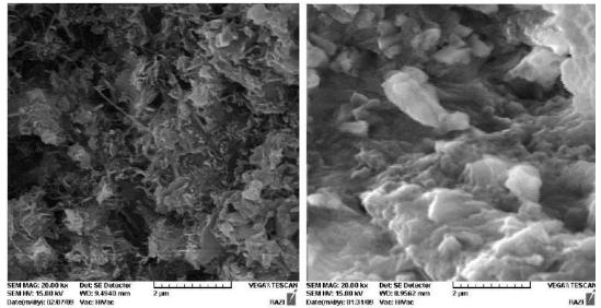
Fig.1:SEM of OPC Concrete & SEM of Nano Silica Concrete (Source: Mostafa.Khanzadi et al.(2010))
