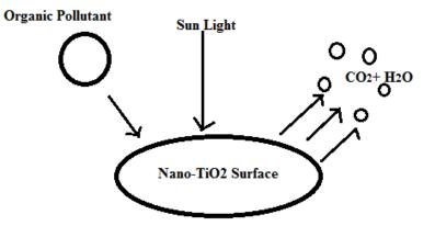
Fig2: Photo catalytic phenomena at Nano TiO<sub>2</sub> Surface
