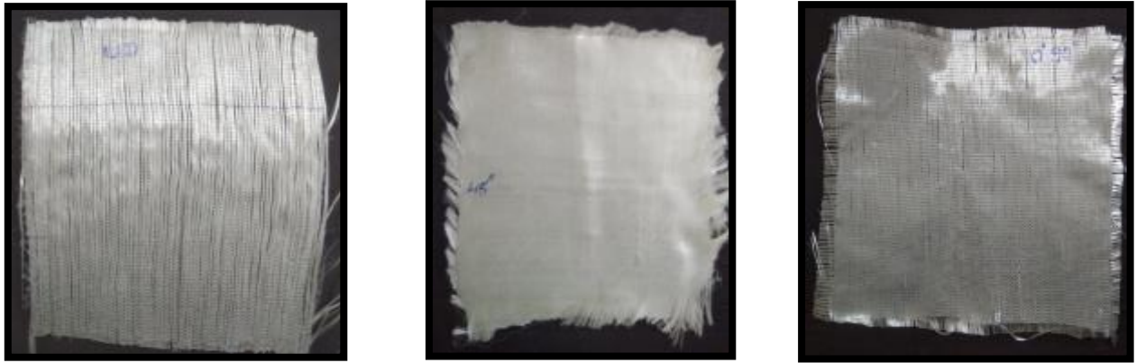
Figure 2. E-Glass fiber [\pm 45^\circ],[0/90^\circ] and Unidirectional
