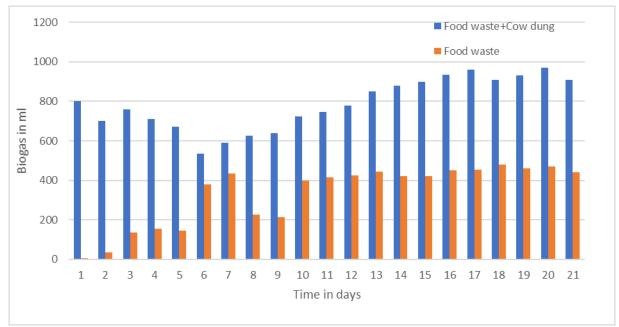
Fig 6. Production of biogas with time
