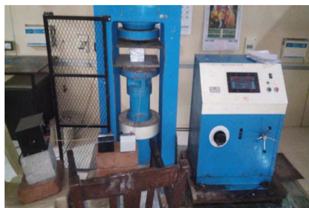
Fig. 2 Compression Test on Cube
