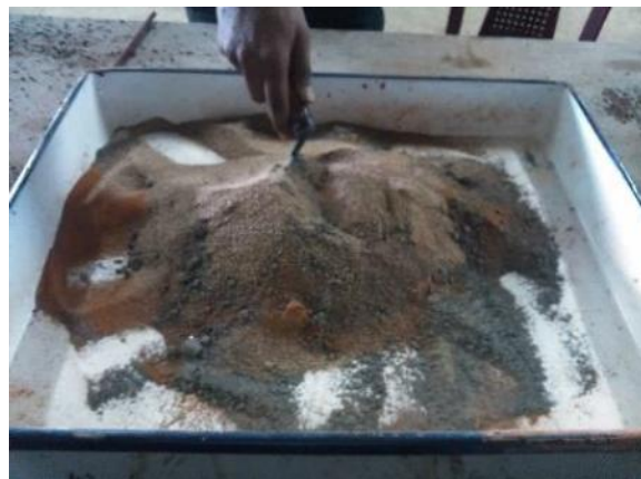
Fig 4.1 Mixing of clay, sand and DAP
