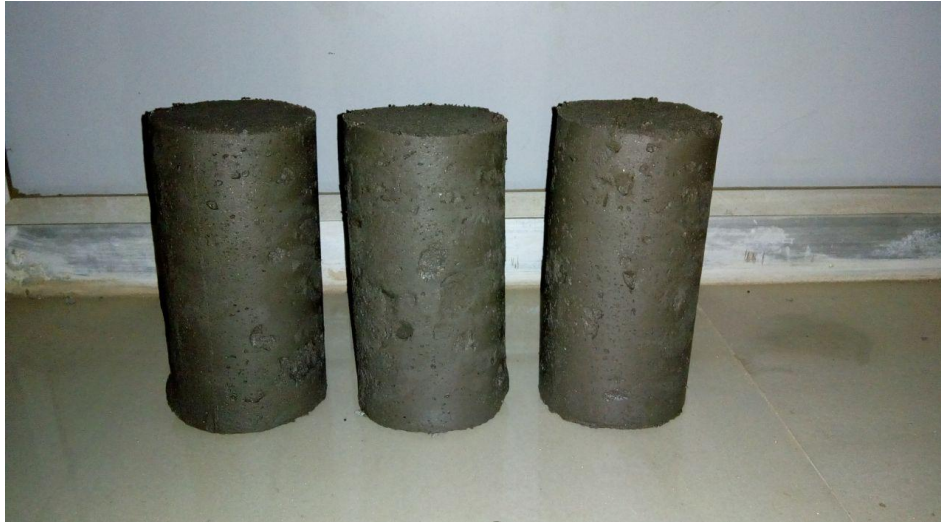
Fig 4.3 Air dry curing under shade
