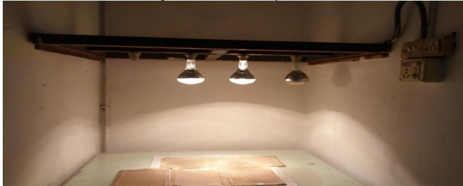
Figure 3. Infrared dryer used for drying mulberry and lemon grass leaves
