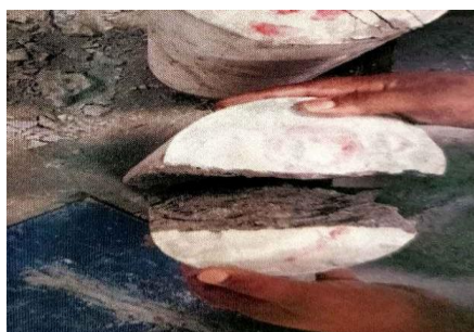
Fig.2 Test specimen after failure (Nominal concrete)
