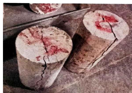
Fig.3 Test specimen after failure (2% steel fibres)
