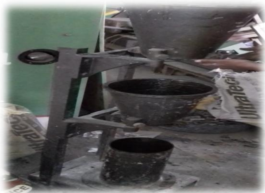
Figure 7: Shows compaction factor test
