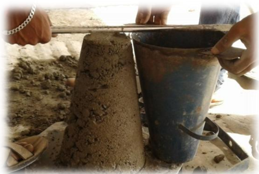
Figure 6: Shows Slump cone test
