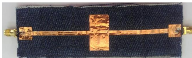
Figure 3- Top view of textile based microstrip low pass filter
