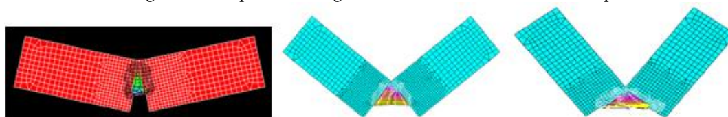
(a) load step no 30 b) load step no 150 c)load step no 400 Fig 9.a: Crack pattern in large notched beam at different load steps
