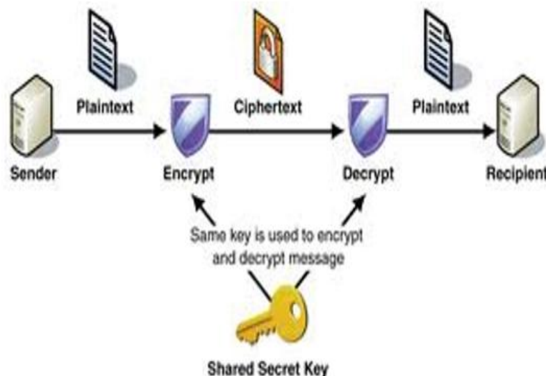
Fig. 1 Diagrammatic representation of symmetric key cryptography.
