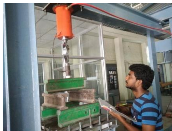
Plate 7: Testing arrangement of slabs for Flexure strength
