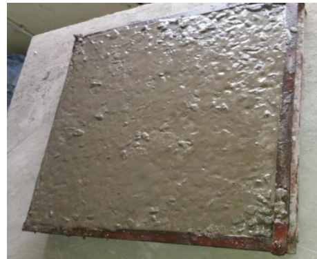
Plate 4: slab mould filled with concrete
