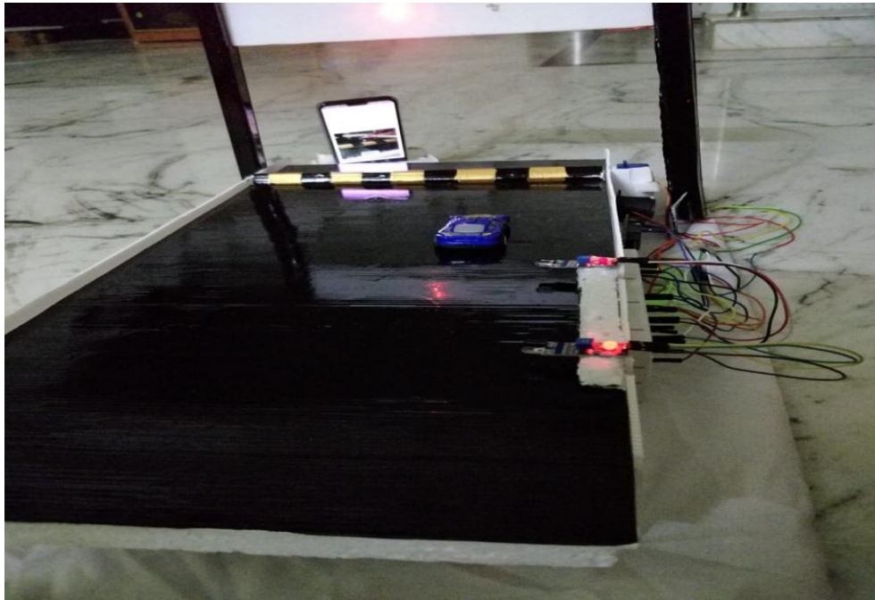
Fig 5.2 : Shows the implementation of the breaker by displaying the red light as the vehicle is over speeding and raising the breaker above the road surface.
