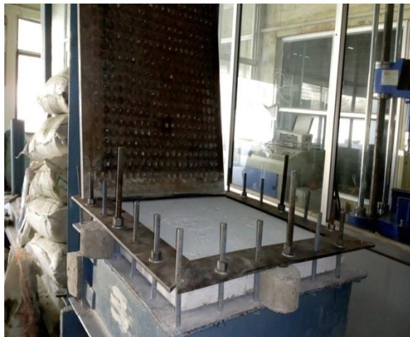
Fig 5: Slab Testing Machine with Fixed Plates
