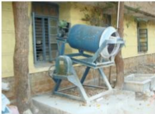
Fig 1: Manufacture process of silica fume aggregate
