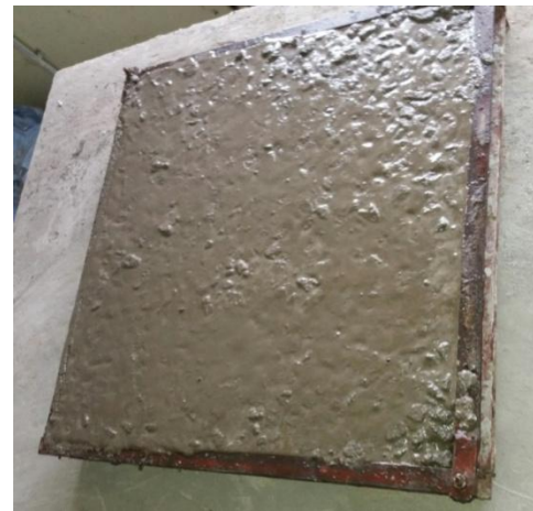
Fig 4: Slab mould filled with concrete
