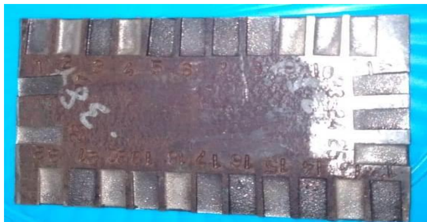
Fig.4: C71500 work piece after machining
