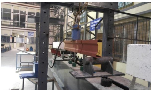
FIGURE 14. EXPERIMENTAL SETUP OF TYPE 3 CONNECTION
