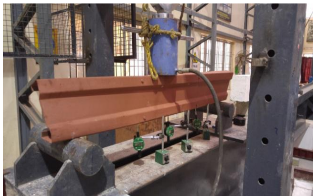
FIGURE 14 FLEXURE-TORSIONAL BUCKLING FAILURE (TYPE 3)
