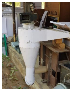
Fig. 2. Experimental setup of vertical cone cyclone separator
