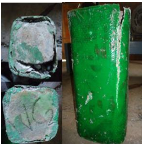
Fig: 8 Failure mode of GFRP concrete prisms
