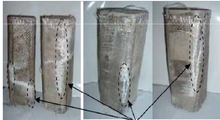
Fig: 5 Failure mode of CFRP confined Cylinders specimens confin
