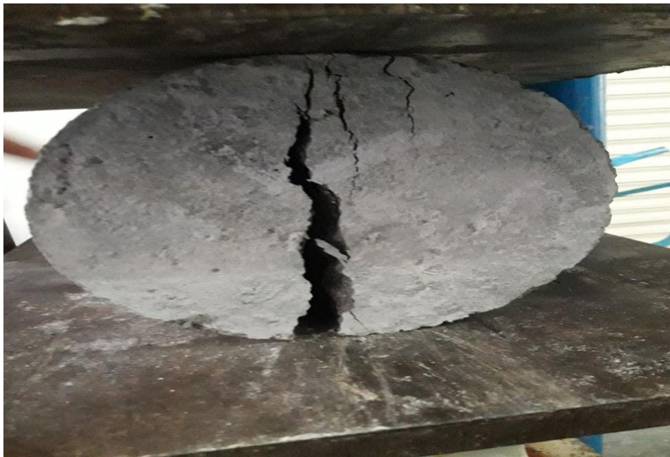
Fig:7 Split Tensile strength test in Compression Testing Machine
