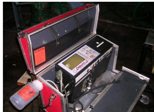
Fig 7: MRU Emission Monitoring System
