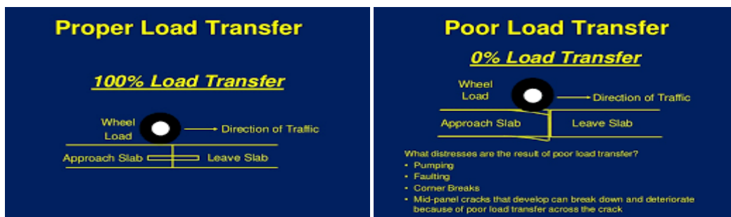
Fig 4.3. Load Transfer Mechanism
