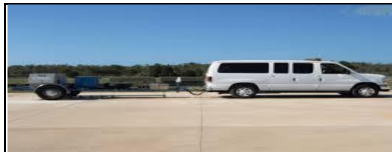
Fig 4.1 Heavy Weight Deflectometer (HWD)
