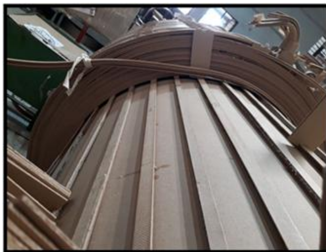
Fig. 3. Transformer cooling ducts.
