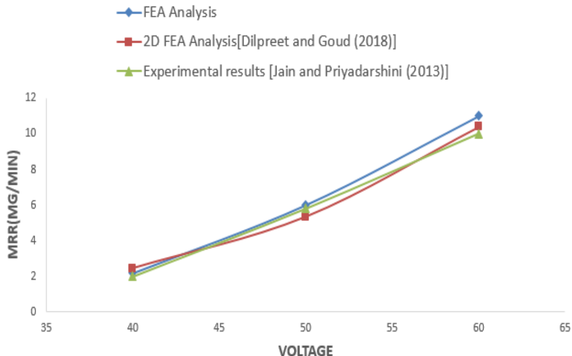
Figure 4.3 comparison of MRR from FEA analysis with MRR from experimental results (Jain and Priyadarshini [18] (2013) and Mudimallana Goud [19])
