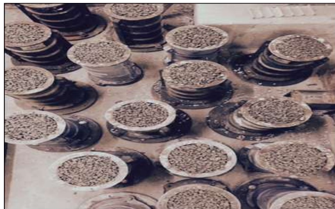
Figure. 1 Photographic view of casting of specimens of pervious concrete mixes in laboratory
