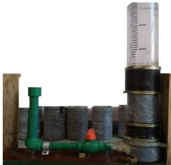
Figure. 2 Photographic view of falling head permeability apparatus used for determining permeability of samples
