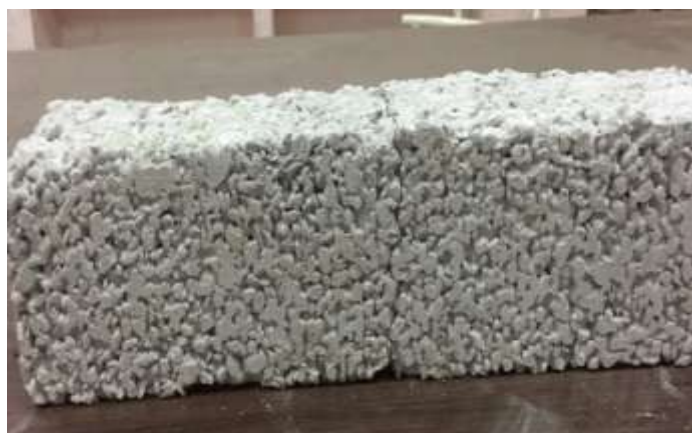
Figure. 5 Failure path of beam specimen after flexure testing
