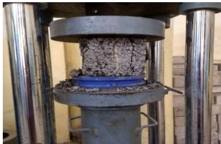
Figure. 3 Photographic view of compressive testing of pervious concrete cubes in the laboratory
