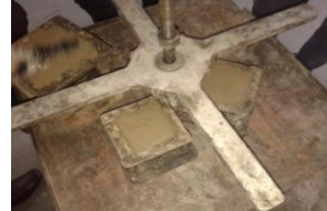
fig. 3.5 Mud mortar cubes on vibrator machine
