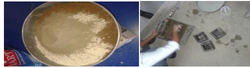
Fig. 3.3 Preparation of mortar mixture
