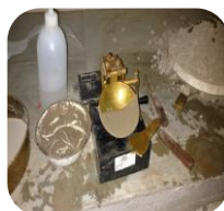
fig.4.4 Liquid Limit by Casagrande Apparatus and
