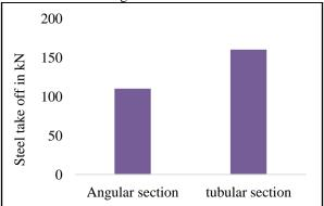
Fig.18 Steel take off comparison of angular and tubular section for K bracing
