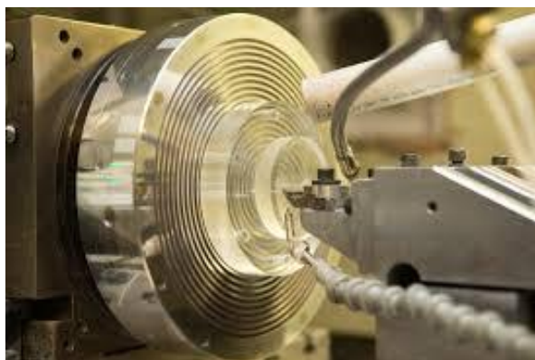
Fig. 2: Single point diamond turning set up
