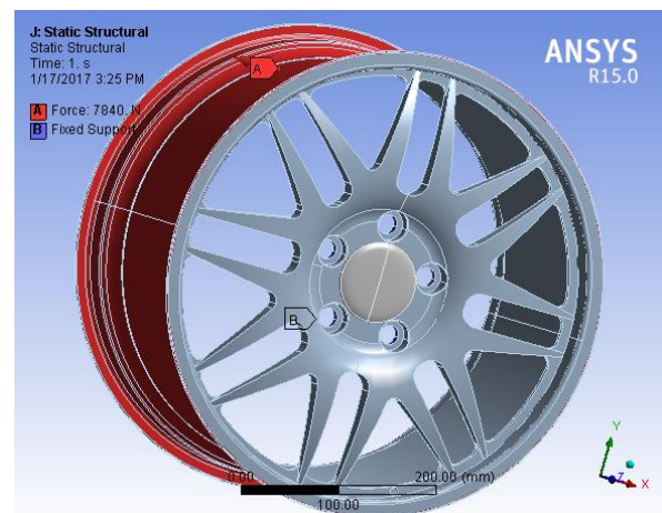
Fig: 4.80 Applying boundary conditions on model 3, A356 aluminium alloy
