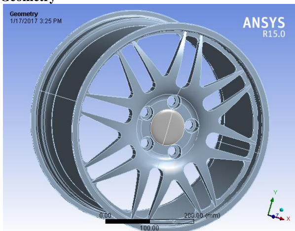
Fig: 4.78 Geometry of model 3, A356 aluminium alloy
