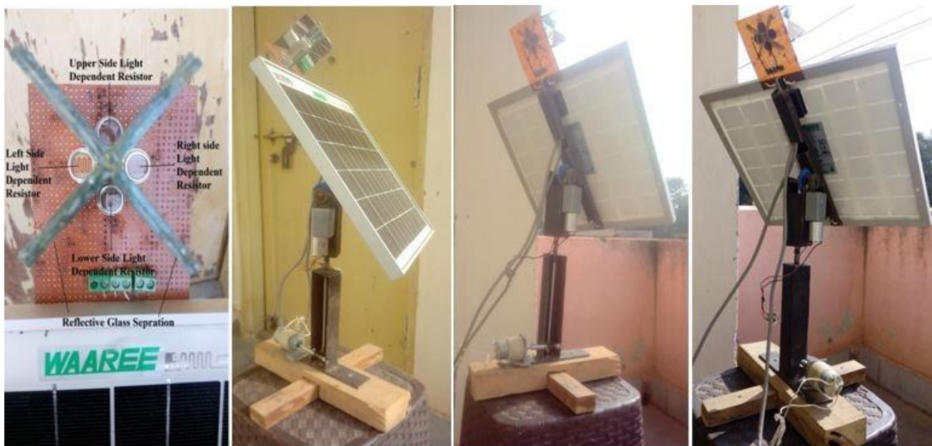
Fig.1 Sun Light Sensing System and Sun Tracking Mechanism
