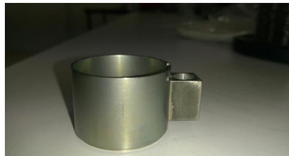
Fig.5 Cover assembly after Brazing
