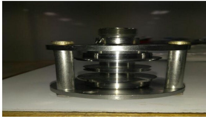
Fig.3 Fixture Mode Assembly of Latch Valve Bobbin
