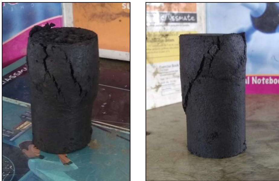
Fig. 2.2 Shear Failure of soil sample
