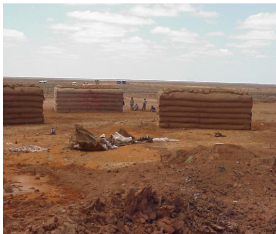
Fig. 09: Mitigation Structures (Source: Field Explosion Test by Kulkarni at Woomera- Australia)
