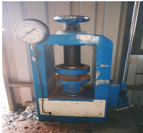
Fig-1: Compression Test of Platic-Sand Brick
