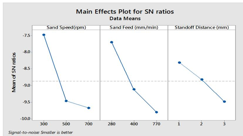
Fig - Effect of machining parameters on Surface Roughness for S/N ratio for Smaller is better
