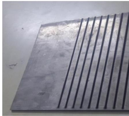
Fig – Final piece with 9 cuts
