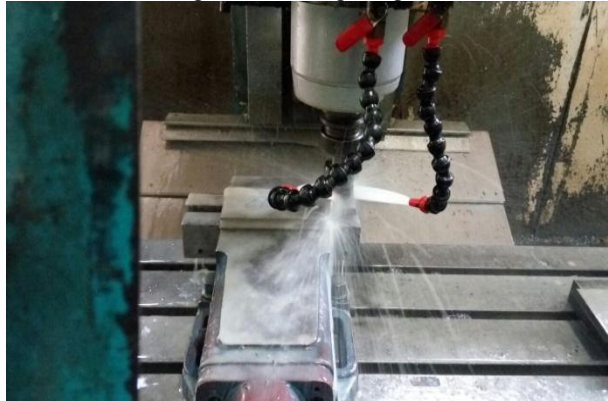
Fig – Machining of work piece by applying parameters – Spindle Speed 1000rpm, Feed Rate – 80mm/min and Depth of Cut – 1mm
