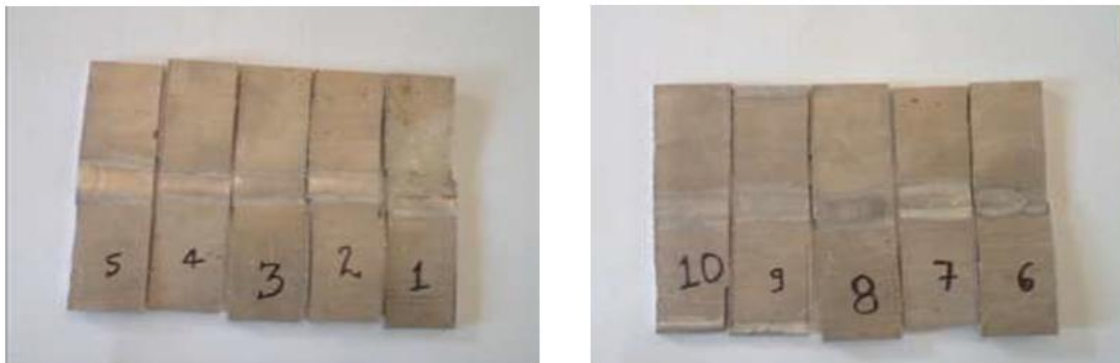
Fig. 4–welded specimen performed with (a) welding speed 3.5 mm/sec & welding current 100, 110, 120, 130 and 140 A are taken for the sample no 1, 2,3,4,5 respectively (b) welding speed 4 mm/sec and welding current 100, 110, 120, 130 and 140 A are chosen for sample no 6,7,8,9,10 respectively
